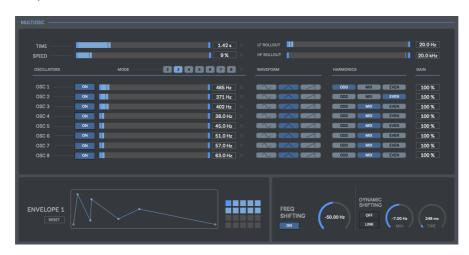
The Multiosc section includes up to 8 oscillators that can generate tones from 20Hz to 6kHz.
